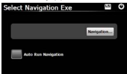
When you have several Navigation maps in the device, if you choose the "Navigation" icon , you can set up one of Navigation maps ( navigation program files ) , and select the Auto Run Navigation , next time when tapping the "GPS" icon on the main menu, the device will run the selected Navigation software automatically .
