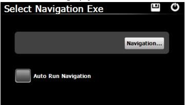
When you have several Navigation maps in the device, you can set up one of Navigation maps (navigation program files) by choosing the "Navigation" icon and selecting the Auto Run Navigation, next time when tapping the "GPS" icon in the main menu, the device will run the selected Navigation software automatically.
